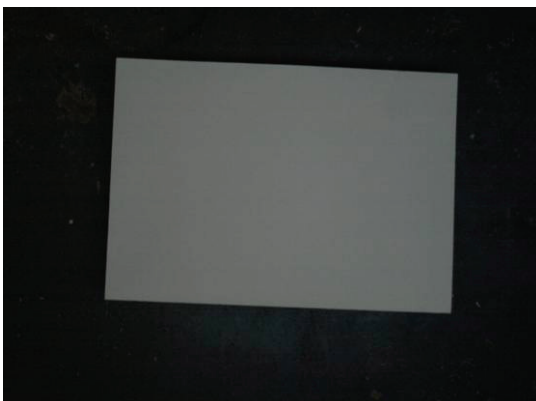
Pictures 5 and 6: Digital top view image of a reference area (paper sheet: DIN A4 = 623.70 cm 2 ) in the box (Picture left) and after modelling by the KobaPlan software (Picture right).
