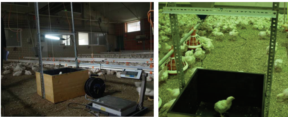
Pictures 1 and 2: Photo box in the broiler barn with metal frame for fixing the digital camera above the broilers
